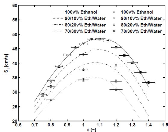
Figure 1: Laminar burning velocity as function of the equivalence ratio of ethanol-air at  $T=318$  K and 1 atm. Lines: San Diego mechanism, Markers: Experiments
